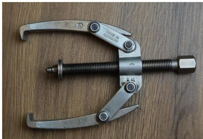
To use this tool the clamps have to be place behind the puller wheel, After this the screw can be screwed forward pushing out the puller wheel. This process is also presented in the picture below.
