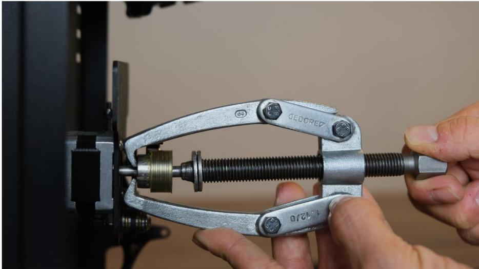
**Step 6:** After the old puller wheel is removed it is time to replace it with a new one. Before placing the wheel it is important to make sure the inside of the wheel is clean. To clean the inside of the wheel it is recommend to press a 5mm drill bit trough such as presented in the picture below.
